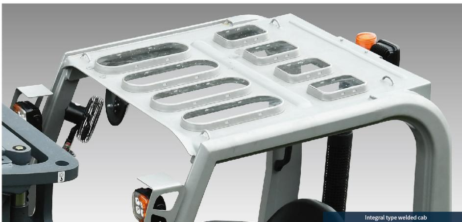
Integral type welded cab
